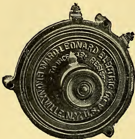
FIG. 240.—The cast-iron plate which forms the supporting structure for the rheostat has several ribs over that part which is close to the resistance wires; the ribs increase the heat dissipating ability of the plate.
